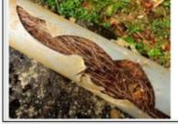
Do ensure all pipe joins are properly sealed to prevent root intrusion
