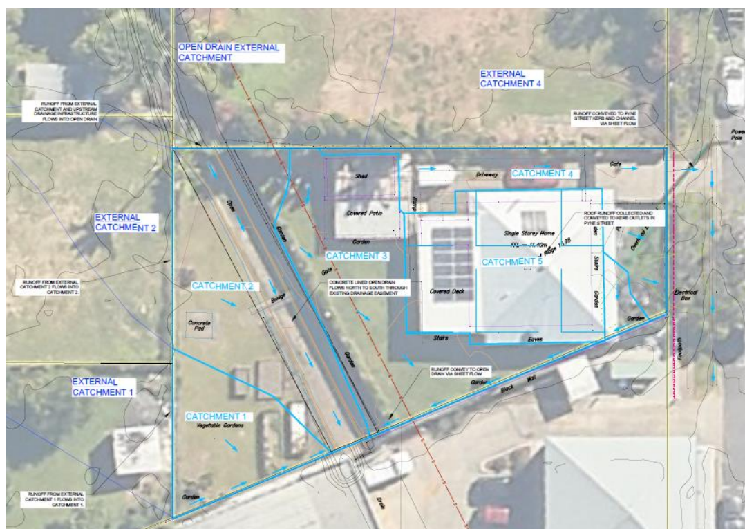
Figure 4: 5 Pyne Street Pre-development Stormwater Catchments
