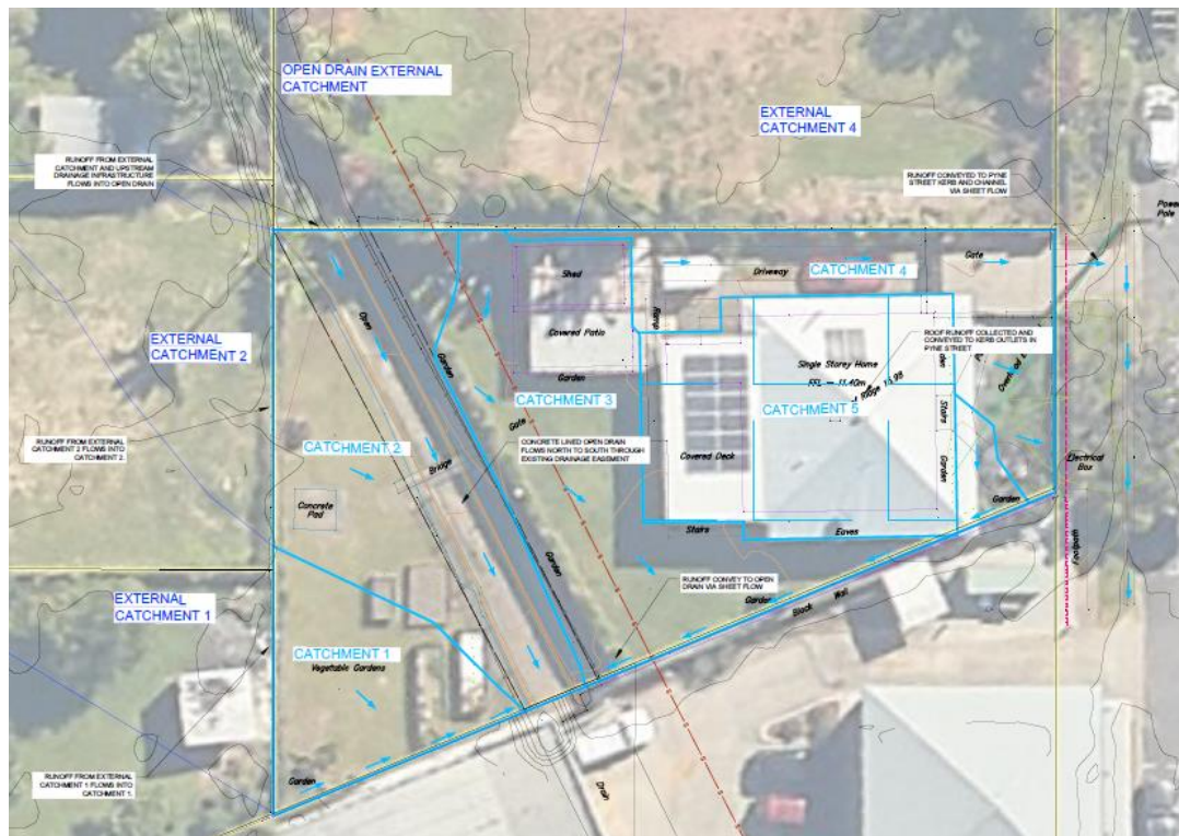
Figure 4: 5 Pyne Street Pre-development Stormwater Catchments
