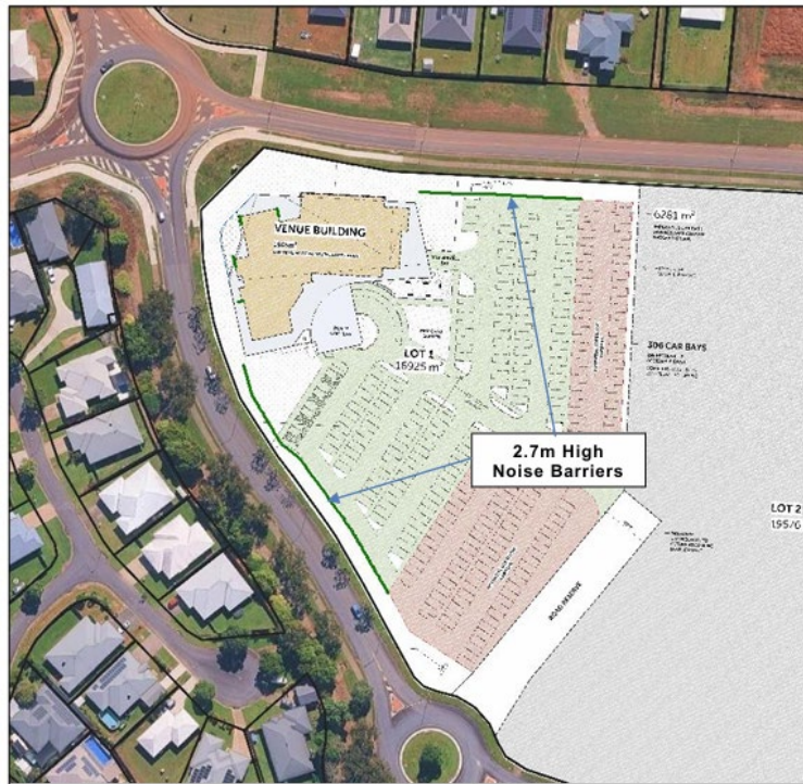
Figure 6.4: Showing recommended noise barrier location
