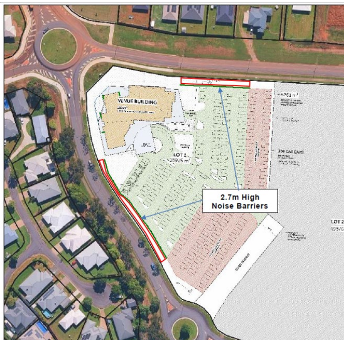
Figure 6.4: Showing recommended noise barrier location
