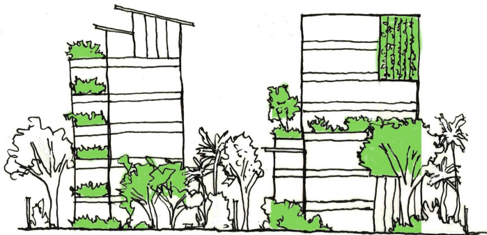
Figure 4.7.b – Front elevation (Landscaping in green is used to calculate vertical landscaping coverage)
