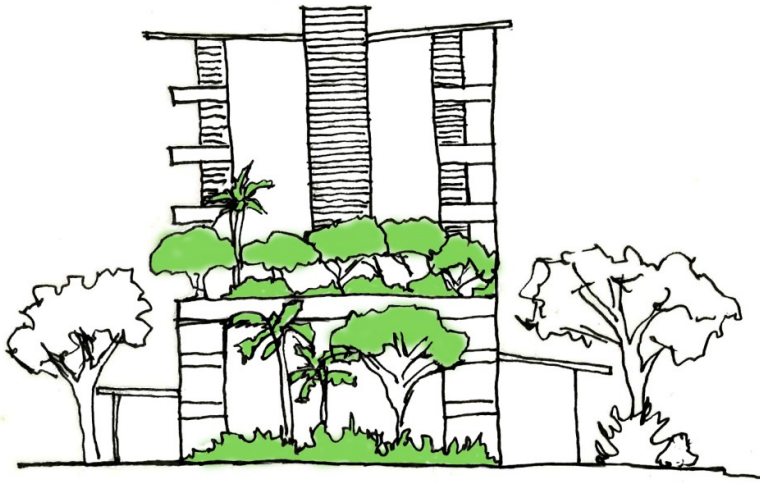
Figure 4.7.c – Side elevation (Landscaping in green is used to calculate vertical landscaping coverage)
