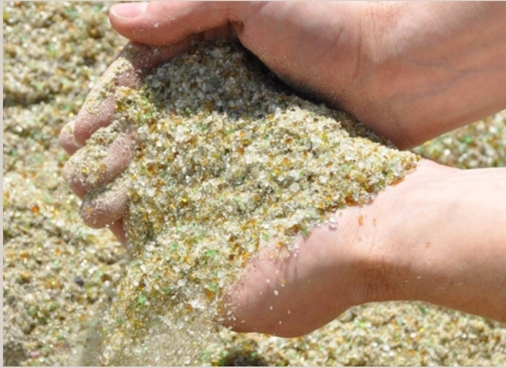
Crushed glass can be used for a variety of applications in civil construction, as a fine aggregate sand replacement or decorative material.
