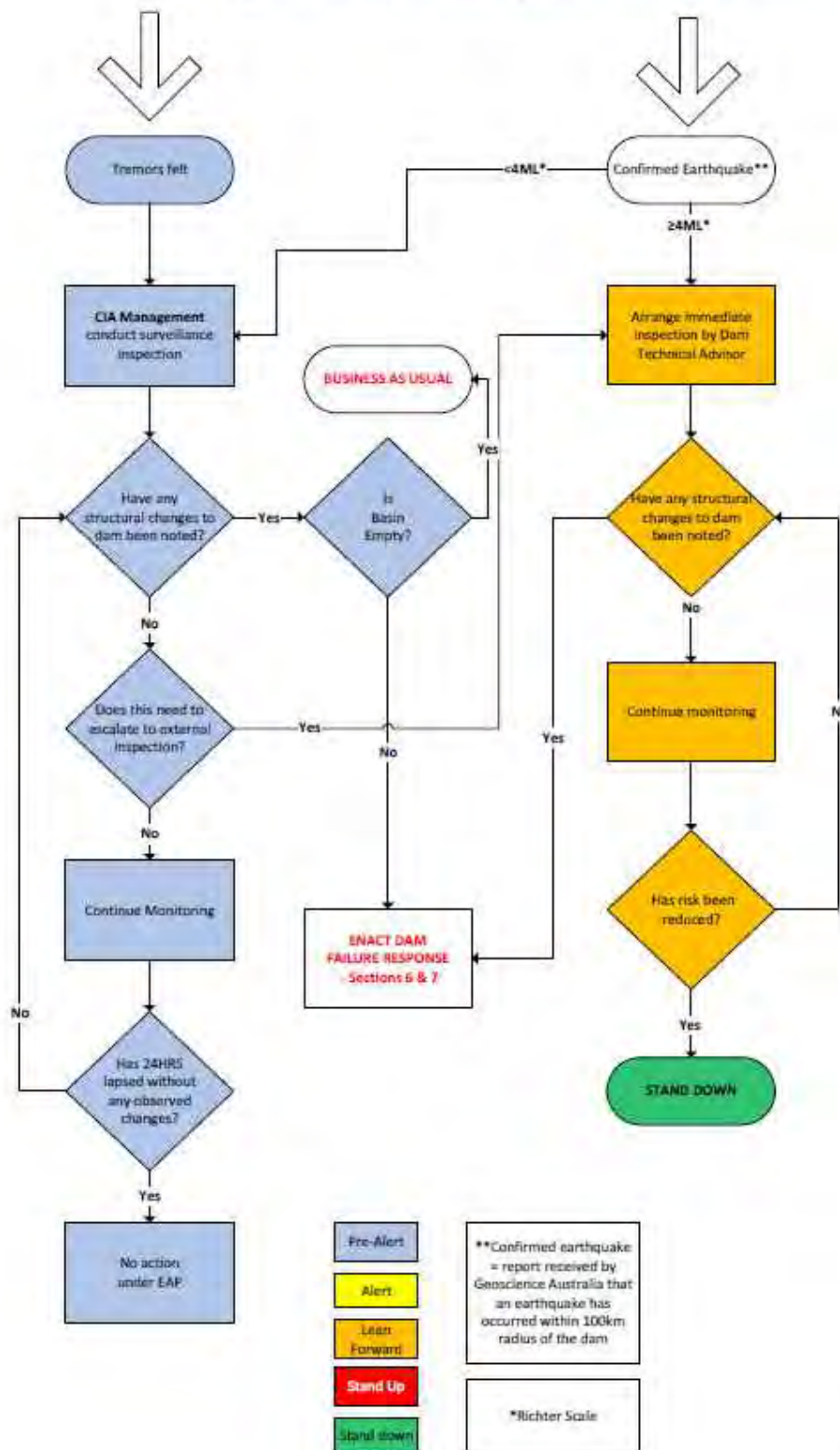
Figure 5: MCB EAP - Earthquake Hazard Flowchart
