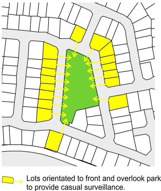
Figure 9.3.8.3.b – Consistent design solution for the orientation of lots surrounding open space and parkland
