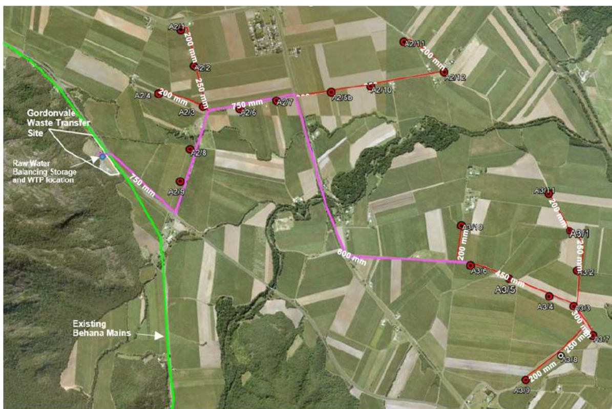
Figure 2: Emergency Borefield and Supporting Infrastructure
