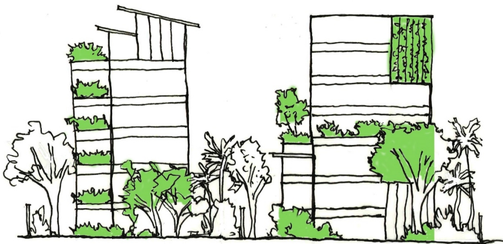
Figure 3.7.b – Front elevation (Landscaping in green is used to calculate vertical landscaping coverage)
