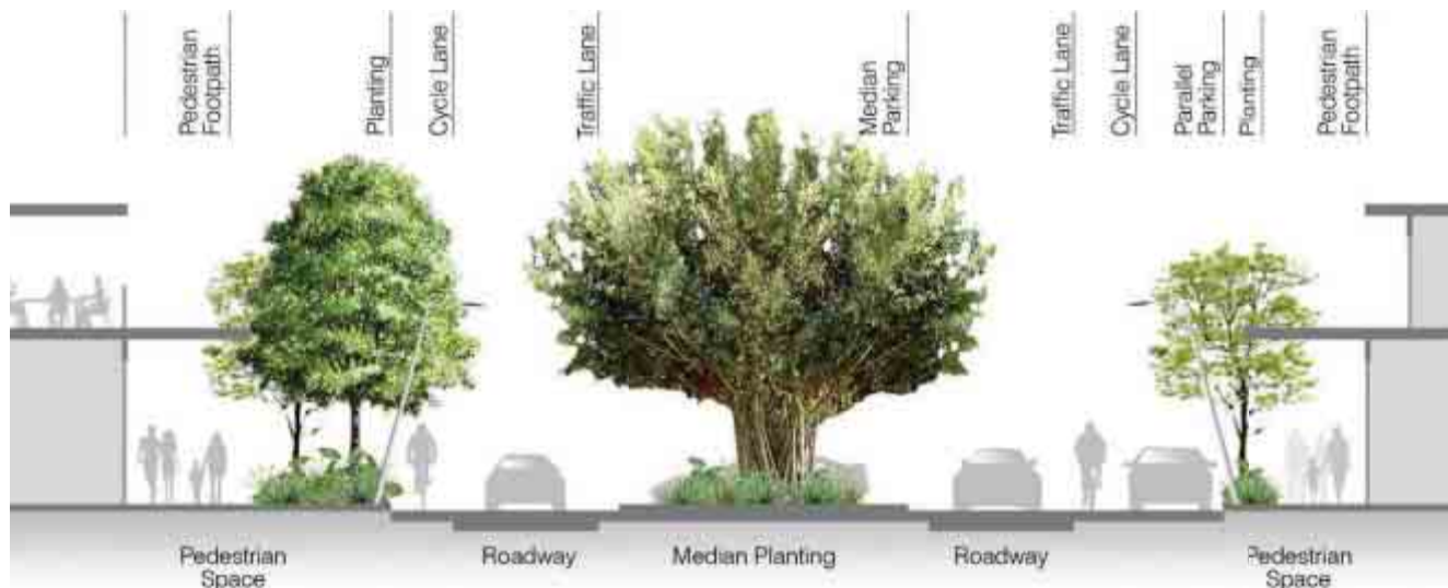
Typical Cross Section - Macrossan Street
