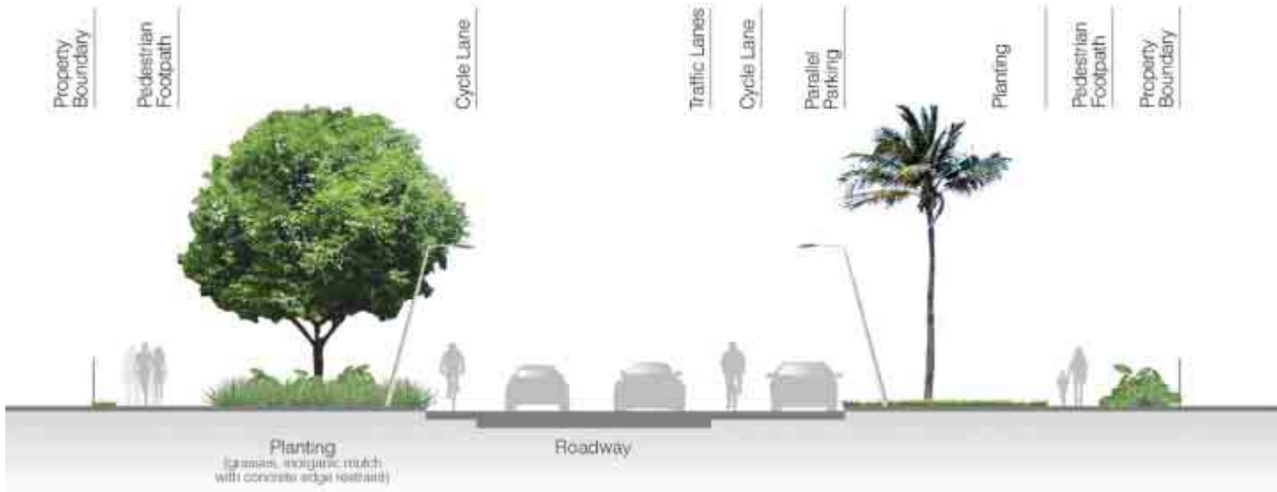
Typical Cross Section - Davidson Street (between Port and Mowbray Streets)
